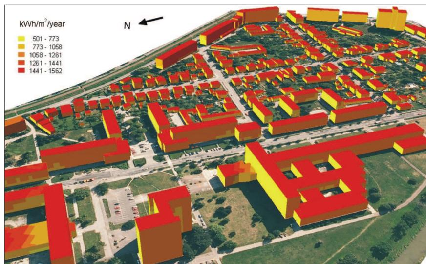
Fig. 4: 3-D solar radiation modelling using the v.sun module
