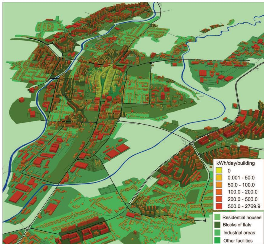
Fig. 3: Assessment of photovoltaic potential in the urban area of Prešov
