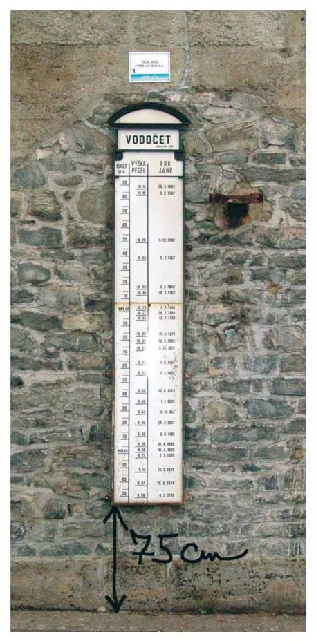
Fig. 9: Water gauge on the Labe River in Ústí nad Labem with the marking of historical floods (Photo: J. Šrejbr). Illustration to J. Munzar's et al. paper
