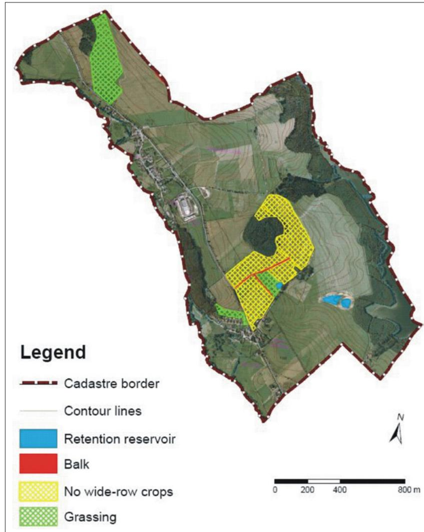
Fig. 2: Soil and water conservation measures realized in the frame of land consolidation
