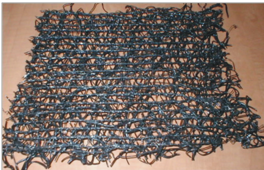
Fig. 3: Sample of one type of spatial geonets, which can serve as a stabilizing element in the body of the slope (photo M. Šlezinger)
