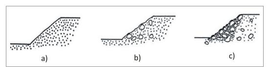
Fig. 3: The stone and soil content of the Form of Anthropogenic Relief: a) muddy, b) muddy-rocky, c) loamy-rocky terraces
