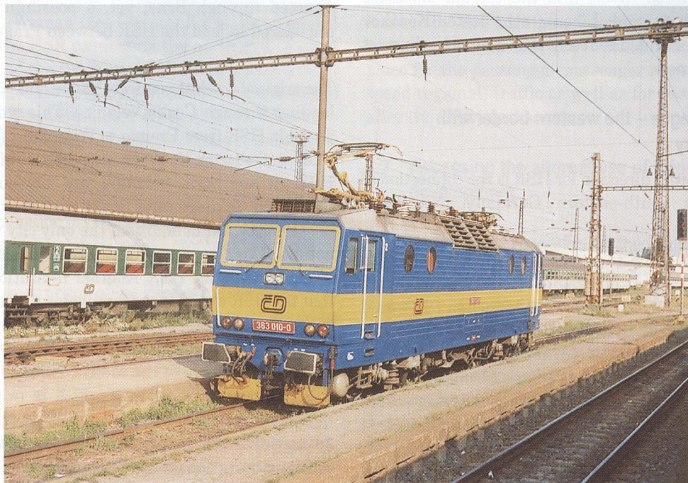
Fig. 5: Two-system engine 363.010 (max. speed 140 km.h -1 ) been used in the Czech Republic most of all for traction of the express trains, railway station Přerov, August 17th 1999. Photo B. Trávníček.
