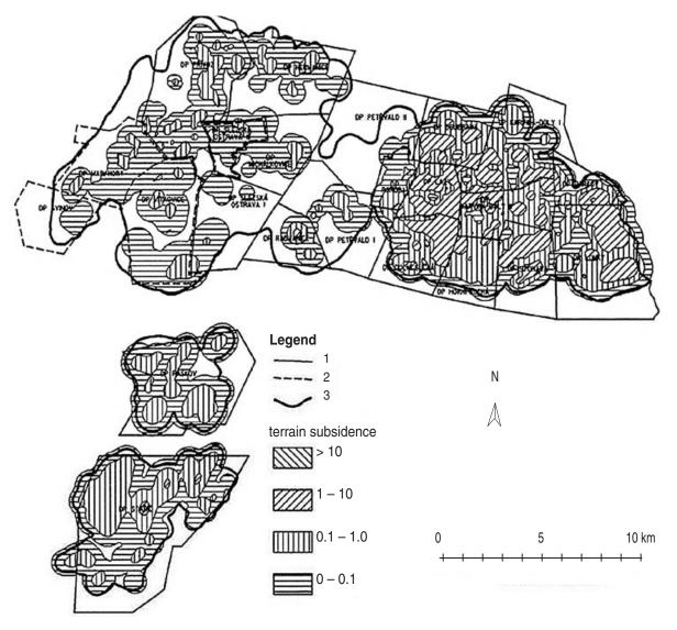
Fig. 3: Isoareas of subsidences from exploitation in 1990 – 1999 Legend: 1 - limits of mine areas; 2 - limits of mine areas with the closed-down mining; 3 - zero subsidence line
