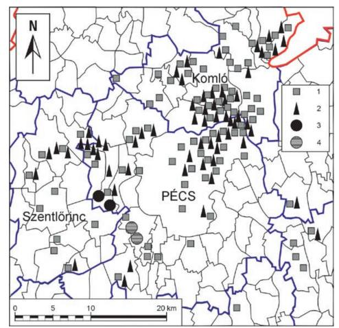
Fig. 2: Environmental damages and danger caused by coal mining in the Pécs-Komló region Legend: 1 – closed mines, 2 – refuse dump, 3 –percolation area of uranium mines, 4 – slurry deposits
