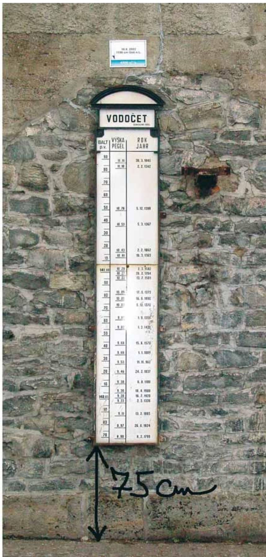
Fig. 9: Water gauge on the Labe River in Ústí nad Labem with the marking of historical floods (Photo: J. Šrejbr).
