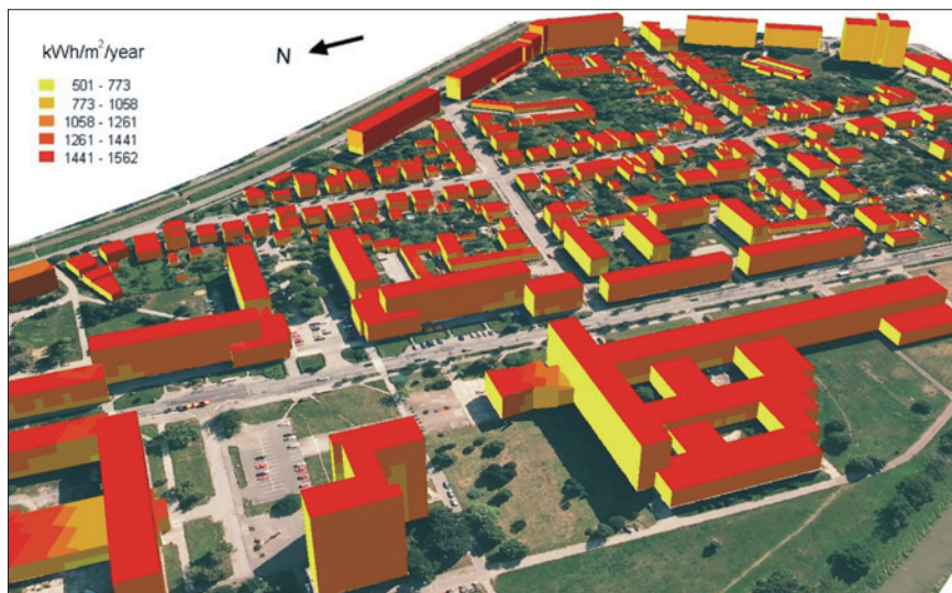
Fig. 4: 3-D solar radiation modelling using the v.sun module
