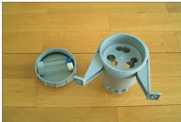
Fig. 2: Diffusive samplers and shelter (Photo: M. Ogrin)
